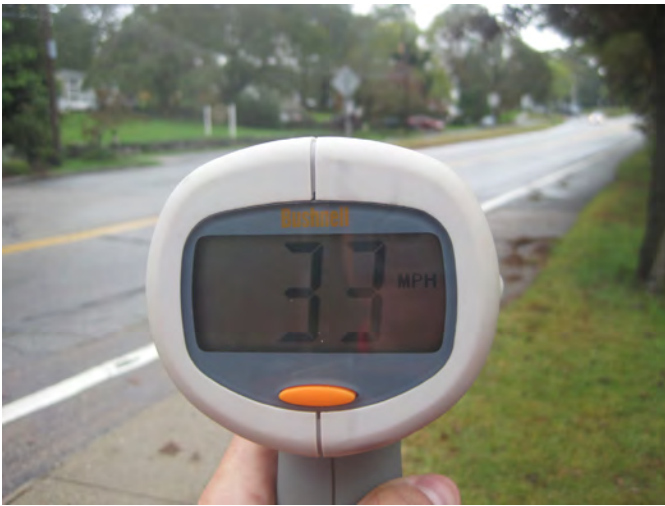
Posted speed limits (25mph) are ignored when the design speed of the road allows motorists to feel comfortable traveling at higher speeds.
